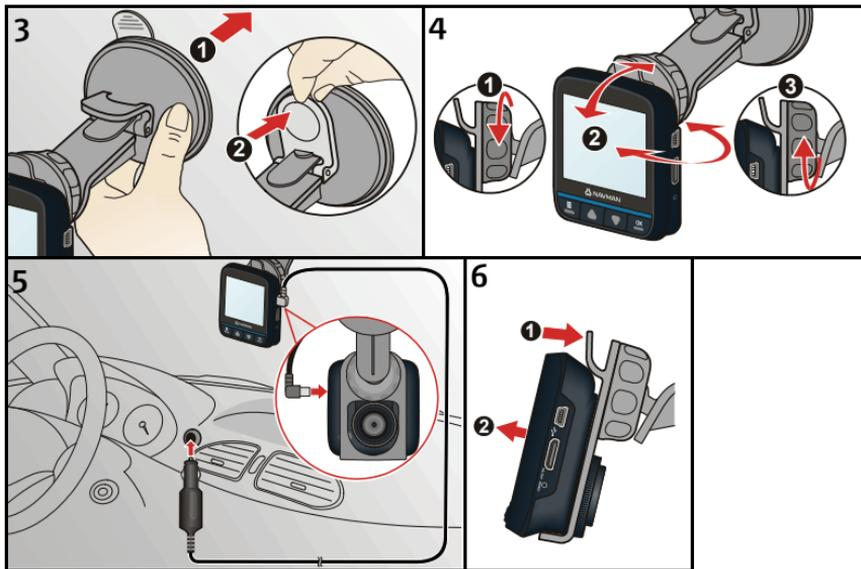
Use cable clips to secure the power cord so that it does not interfere while driving. To ensure the highest quality recordings, you are advised to place the recorder near the rear view mirror.
